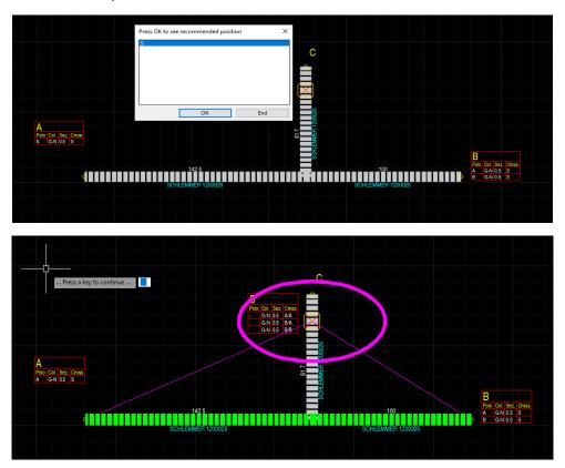
In the example, the position of the S1 splice would be in a more correct position if it were inserted in the horizontal paths because none of the connections related to the splice involve group C. This case is elementary, but on complex harness such as the automotive one, this tool will be extremely important.
