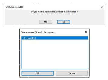
By pressing OK you can see the Bundles of the selected Harnesses. This command is very useful for correctly drawing the harness or harnesses before proceeding with the insertion or import of the Groups at their ends.
