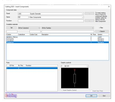
The next dialog box allows you to combine the Pins of the Component with the Pins of the Group. It is not allowed to insert complex components with multiple Ports.
