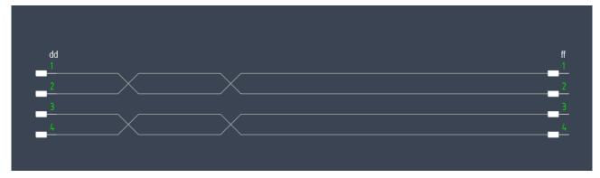
In the presence of the Connection Indications, if they are found in the twist area interval, they are automatically deleted.
