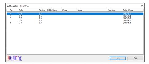
This allows you to insert the Pins in the desired order also based on their connections: for example, if the connections are twisted, you can draw them close together as they will facilitate the representation of the twists on the connections.
