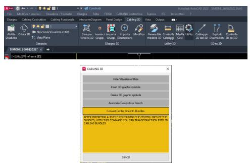
In fact, CABLING warns that the conversion of the Center Lines must be done on a layer with a name starting with 'Axis\_ \*' (for example Axis\_1).
