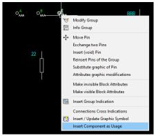
This new option opens the Component insertion dialog box where you can choose the Component and enter the name and function.
