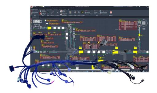
CABLING has in fact created a market standard used by both producers and designers of harnesses because it offers all the information necessary for both the production and the realization of the technical documentation. Drawings can be shared between companies or between departments of the same company, creating synergy and reducing time and errors.
