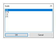
With the command CABLING Wiring Diagram  $\rightarrow$  Wiring Diagram Utilities the new scale is requested and CABLING performs the scale maintaining the same standards as regards the connection indications.
