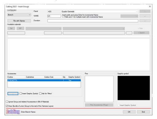
In fact, the Accessories area, previously frozen, is now active allowing you to choose the desired accessories that will be inserted as visible accessories and matched to the branch node. For this reason, if an accessory does not have An associated graphic symbol it cannot be inserted and the following message is returned:
