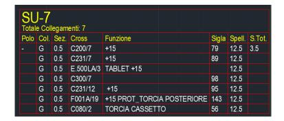
The 'Total Connections' is inserted at the top of the table with the information of how many Connections the Group has, whatever type it is.
