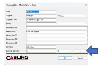
The new button has been added [...] indicated by the blue arrow which opens a new window where you will have the list of the main sections in mm2 with the corresponding external diameter. These are theoretical data typical of the automotive sector and must be verified with the actual type of wire which may have diameters depending on the type of insulation.
